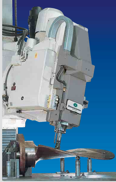
Vertical milling head with \pm 90^\circ continuous swivel B-axis.
