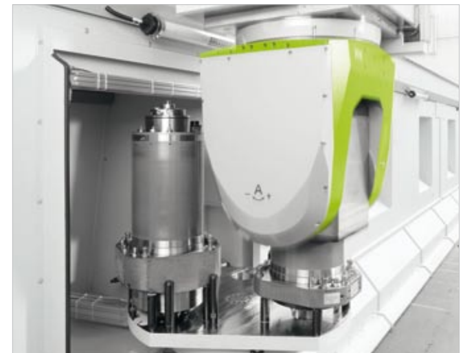
Spindle station embedded in the side wall for the fully automatic spindle change of up to three spindles.
