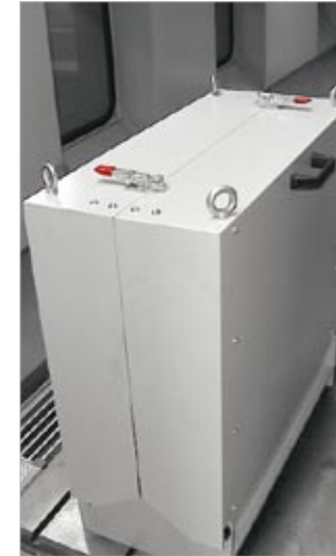
The mobile spindle change box for semi-automatic spindle change (option).
