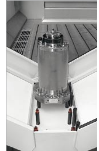
Spindle stored in the mobile spindle change box, ready for semi-automatic change.
