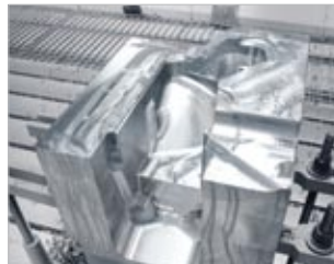
Heavy roughing operations even in the tool and die industry for perfect dies and moulds.
