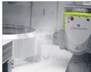
Heavy roughing and finishing operations of titanium in one set-up utilizing the spindle exchange system MuST®.
