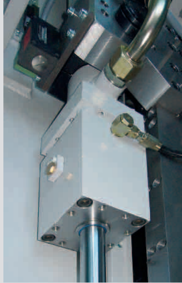
▲ Strong clamping head for effective protection of the Z-axis in case of power failure.
