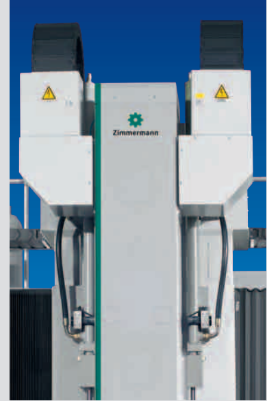
▲ The Z-slide – extremely rigid design while still light in weight.
