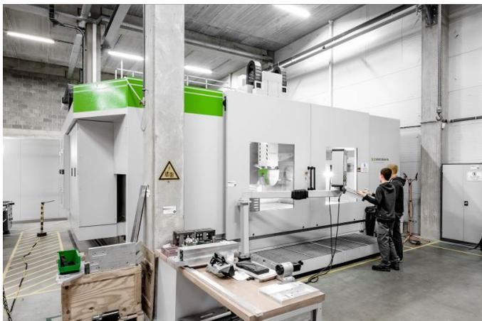
**Figure 6:** For this purpose RapidFit relies on a portal milling machine FZ33 compact from F. Zimmermann GmbH.
