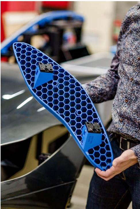
**Figure 4:** The components are manufactured by additive 3D printing from aluminium, polyamide or specially developed materials.
