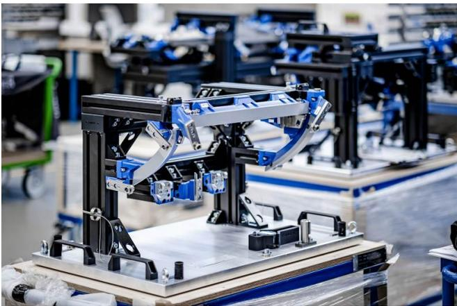
**Figure 8:** Jigs, gauges and fixtures are part of the Smart Cube.
