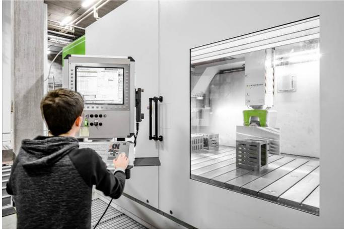
**Figure 5:** In order to achieve a very high accuracy of the parts, they are mechanically finished.
